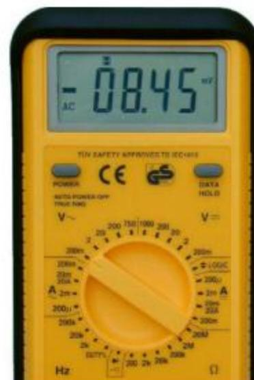
**TENSION AC** 200 mV, 2, 20, 200 V  $\pm 0.5\% + 10d$  10-100  $\mu V$ -1-10 mV
